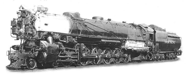
The version next is the 'as built' UP-2 class equipped with the 'BL' style feedwater heater hung on the fireman's side of the locomotive, a very distinctive look. This group included road number 9001-9014
